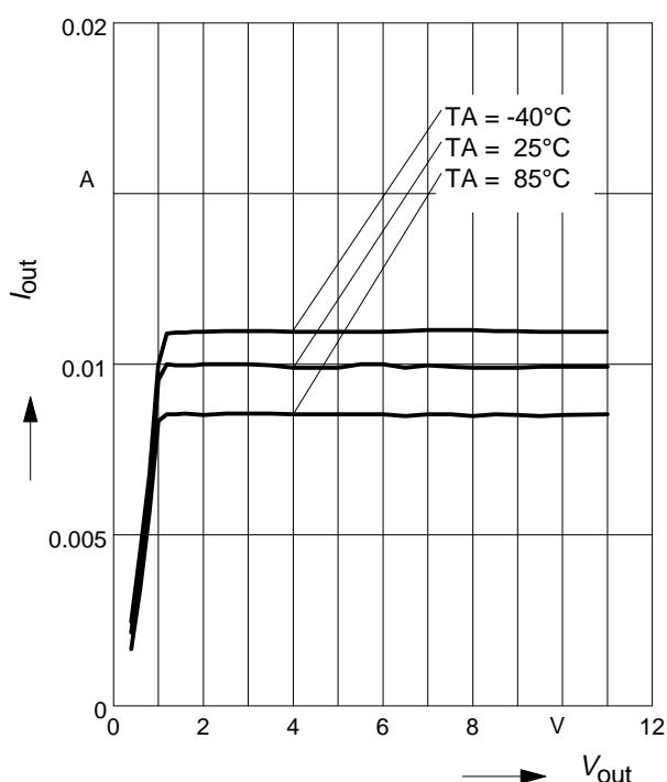
**BCR320U: Output current versus  $V_{out}$**
