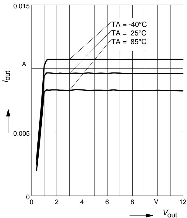
**BCR321U: Output current versus  $V_{out}$**
