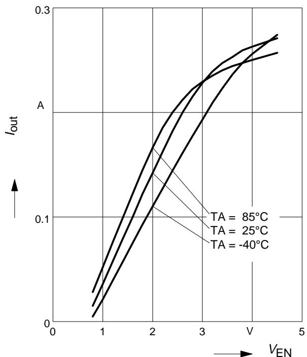
**BCR321U: Output current versus  $V_{EN}$**
