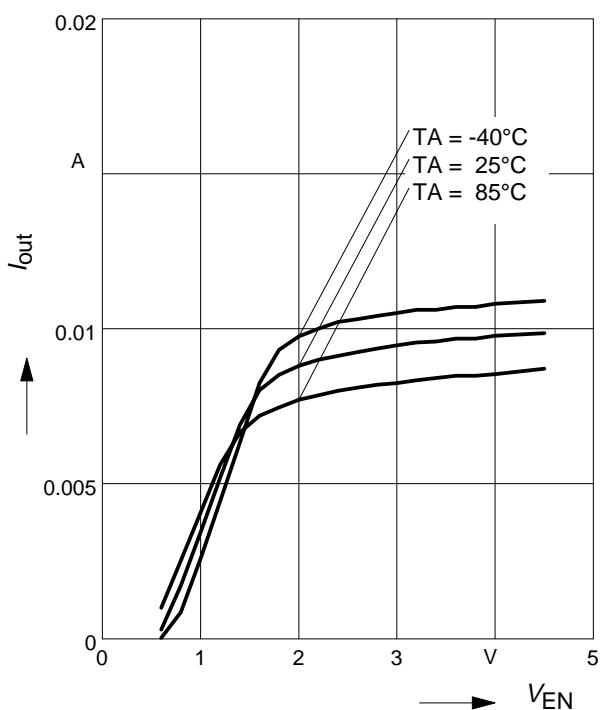
**BCR321U: Output current versus  $V_{EN}$**
