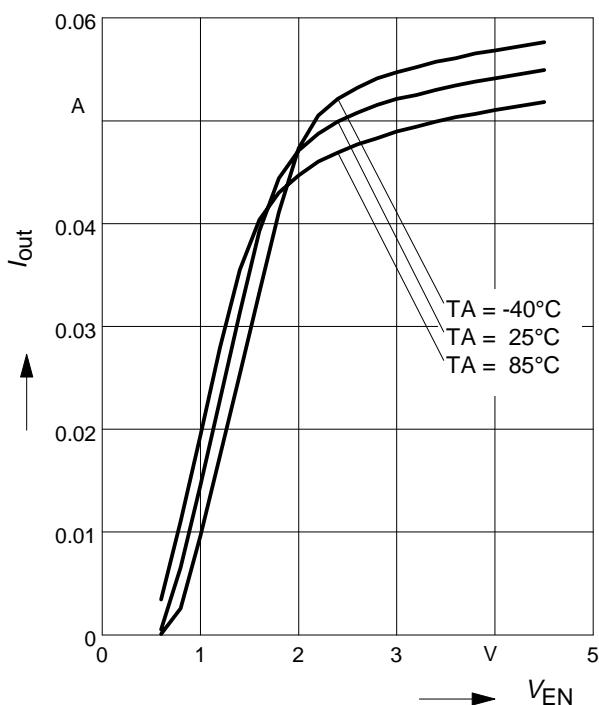
**BCR321U: Output current versus  $V_{EN}$**
