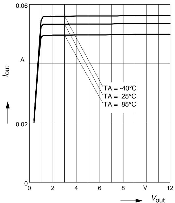
**BCR321U: Output current versus  $V_{out}$**
