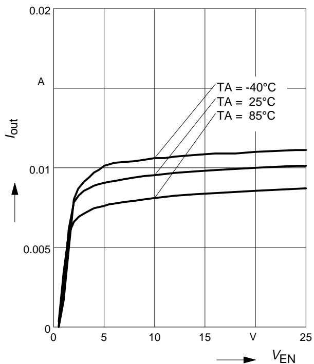
**BCR320U: Output current versus  $V_{\text{EN}}$**
