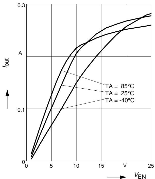
**BCR320U: Output current versus  $V_{EN}$**
