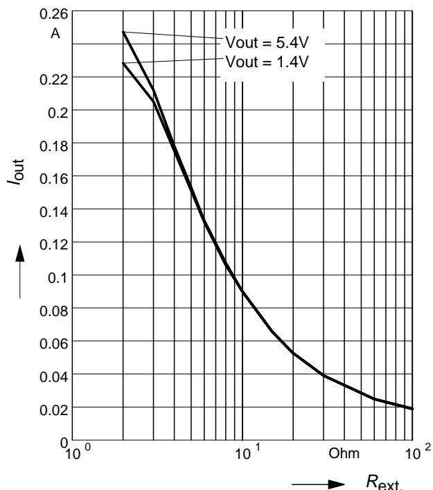
**BCR320U: Output current versus  $V_{out}$**
