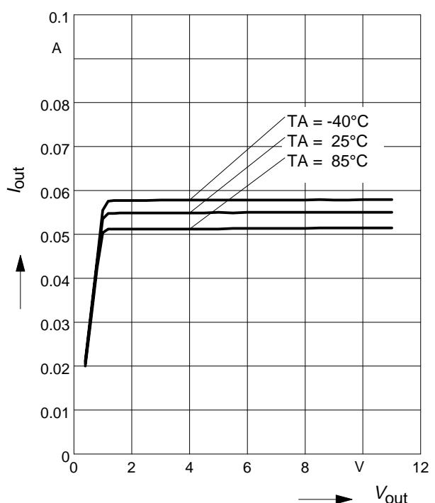
**BCR320U: Output current versus  $V_{\text{out}}$**
