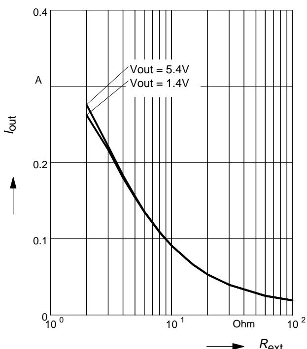
**BCR321U: Output current versus  $V_{out}$**
