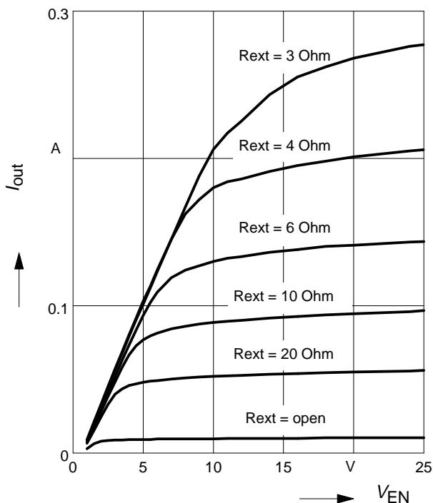
**BCR320U: Enable current versus  $V_{EN}$**
