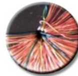
Step 3: Lid fitted & secondary wound around case
